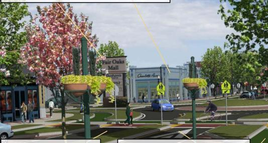
The protected bike lane follows the form of the roundabout, physically separated from the motor vehicle lane and the sidewalk. Vehicles such as the SUV below are facing the bike lane and pedestrian crossing, and are traveling at a slow rate when encountering the crossings, improving safety for all. This type of protection will also increase bicycling and walking rates.
