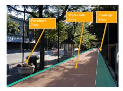
furniture and other materials can distinguish functional areas of sidewalks. When building a sidewalk, contractors should be advised that utilizing trowel cuts, rather than saw cuts, to create a better surface for wheelchairs and wheeled devices.
